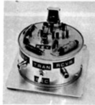
View of the assembled Tuna-Tin 2. Dymo tape labels are used to identify the connectors and switch. The chassis is affixed to a base plate by means of No. 6 spade bolts.
