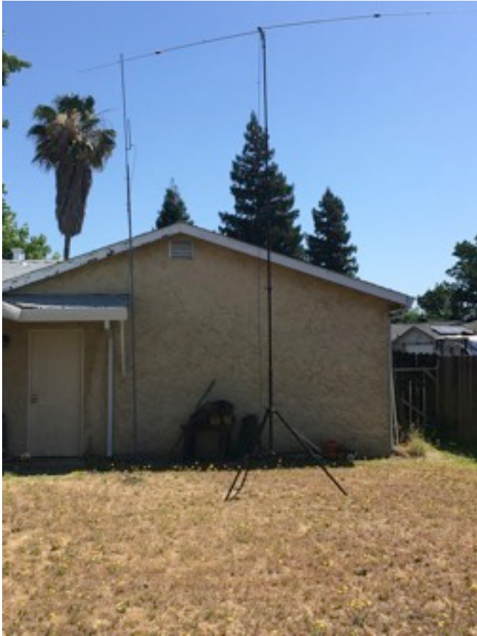
Dipole set up in my back yard for Field Day.
