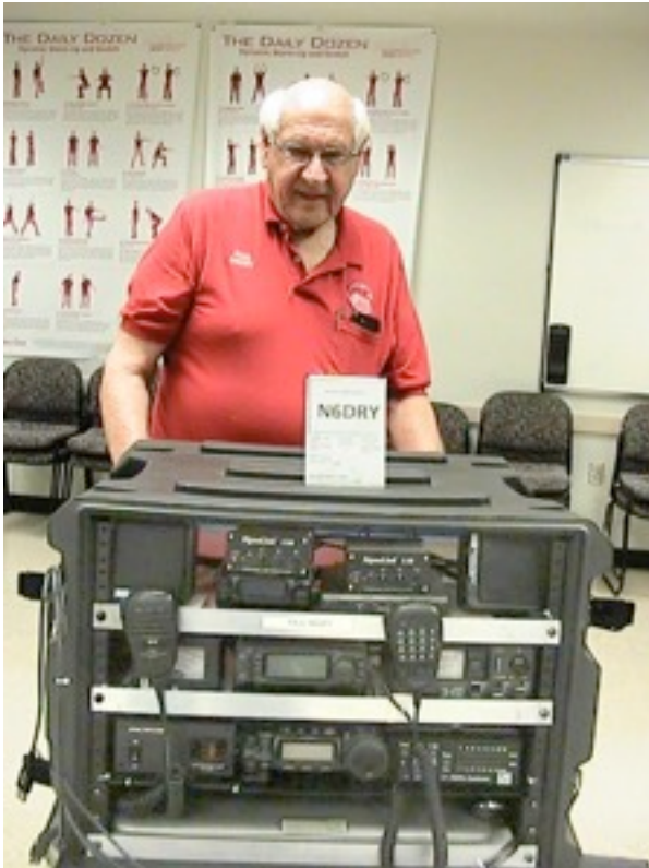
Paul Grose N6DRY repurposed a Transporter Chair and Gator Box for use as a self contained roll around HF, VHF and packet digital data station at an assisted living community.
