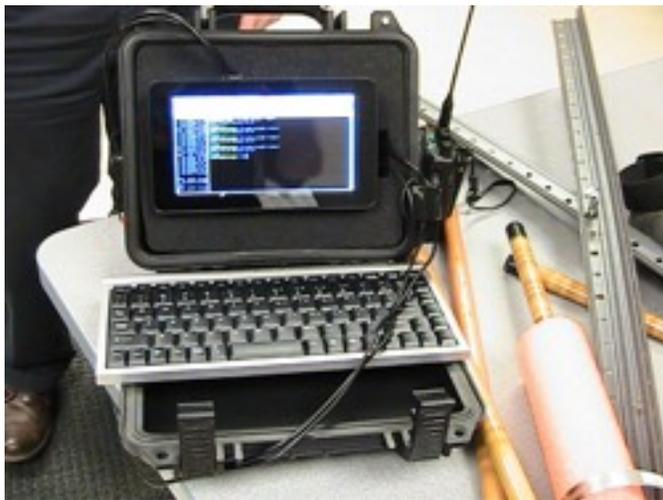
Close up of Kevin Hooke's homebrew portable packet radio station
