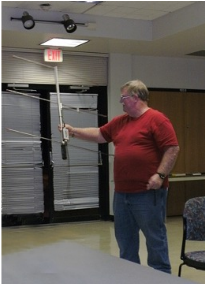
Rick-McCusker WF60 shows a directional antenna with attenuator used in Foxhunting.
