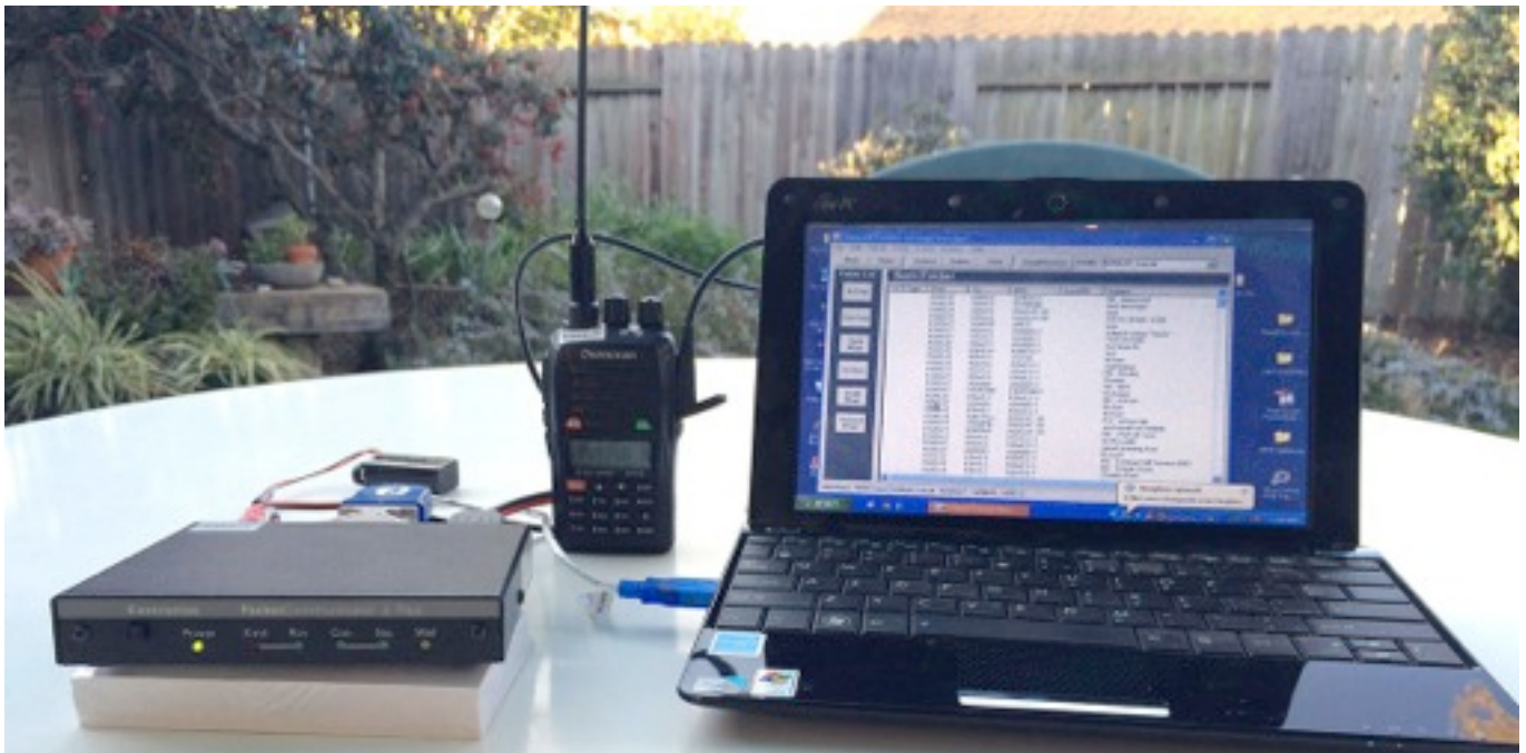
Windows netbook, HT radio, KPC3 TNC, 9v battery USB to serial cable to TNC, radio to TNC cable Outpost Packet manager running on netbook
