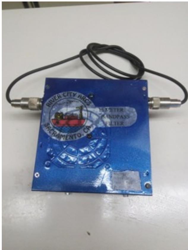
Dave Martin WB6YLK built this 15 Meter Bandpass Filter
