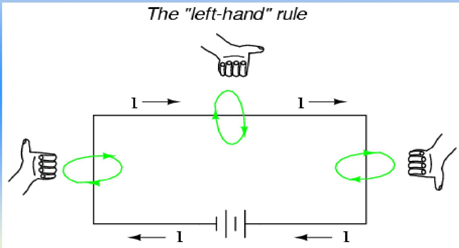
The magnetic field encircles this straight piece of current-carrying wire, the magnetic flux lines having no definite "north" or "south" poles.
