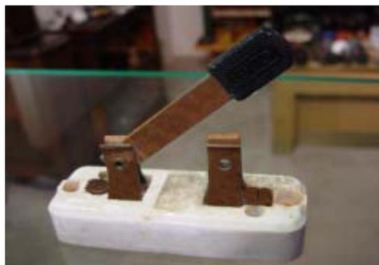
A knife switch is nothing more than a conductive lever, free to pivot on a hinge, coming into physical contact with one or more stationary contact points which are also conductive. The switch shown in the above illustration is constructed on a porcelain base (an excellent insulating material), using copper (an excellent conductor) for the “blade” and contact points. The handle is plastic to insulate the operator’s hand from the conductive blade of the switch when opening or closing it.
