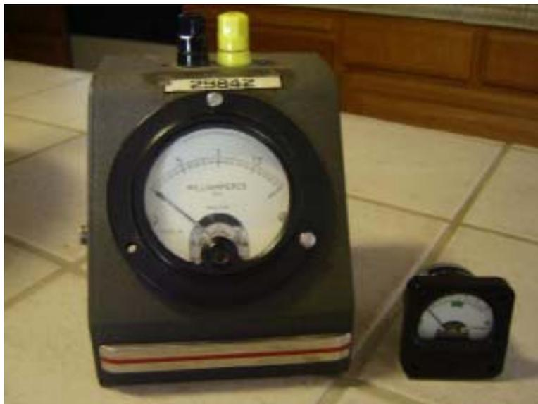
**The meter above is an old Weston “2 ma” meter that will be used as the test “meter” following.**
